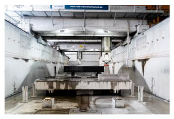
To process such blocks precisely, Reitz relies almost exclusively on machines developed and built in-house: four gantry-type milling machines and two 5-axis gantry machines, all controlled by Siemens 840D. To ensure safe, fast, and precise granite machining, the company uses Vericut simulation software.
